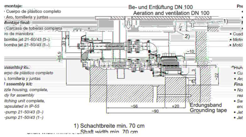
2) Schaltanlage in trockenem Raum montieren Switchboard unit to be installed in a dry location
